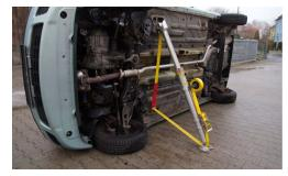
on some rural roadways; the equipment we currently have takes a long time to set up, is cumbersome, and sometimes the wood is too long for what is needed (especially on the roadway). Not having proper or precise stabilization put our firefighters at risk of the vehicle shifting or rolling back over on personnel when not secured properly.
