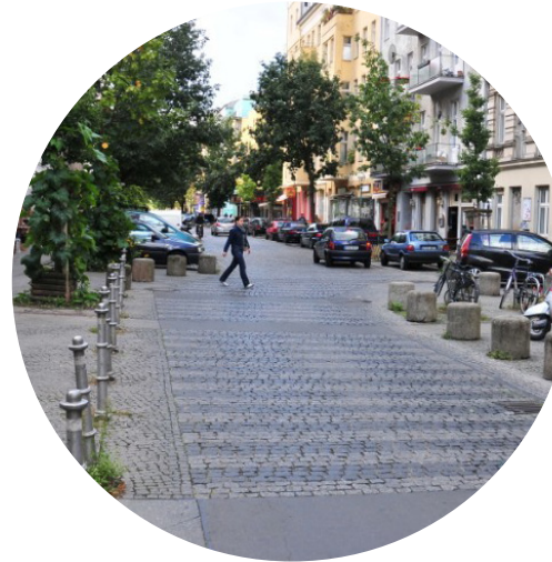
URBAN EDGES: bollards, raised planters, etc. provide buffer between travel zones and amenity zone
